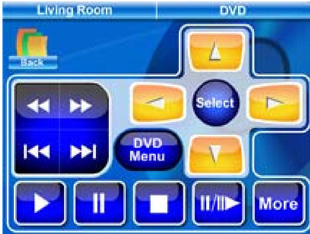
New DVD Player control screen for control of DVD player connected to a MediaLinX MLA101.
