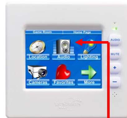
Program the AUDIO button to control a lighting scene.
