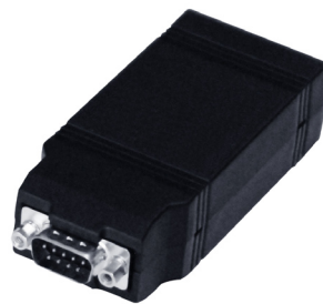
NS-MNE showing RS-232 connector end that interfaces to MU5066ADC
