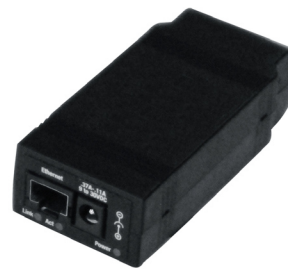
Rotated NS-MNE showing end that interfaces to Ethernet and Power
