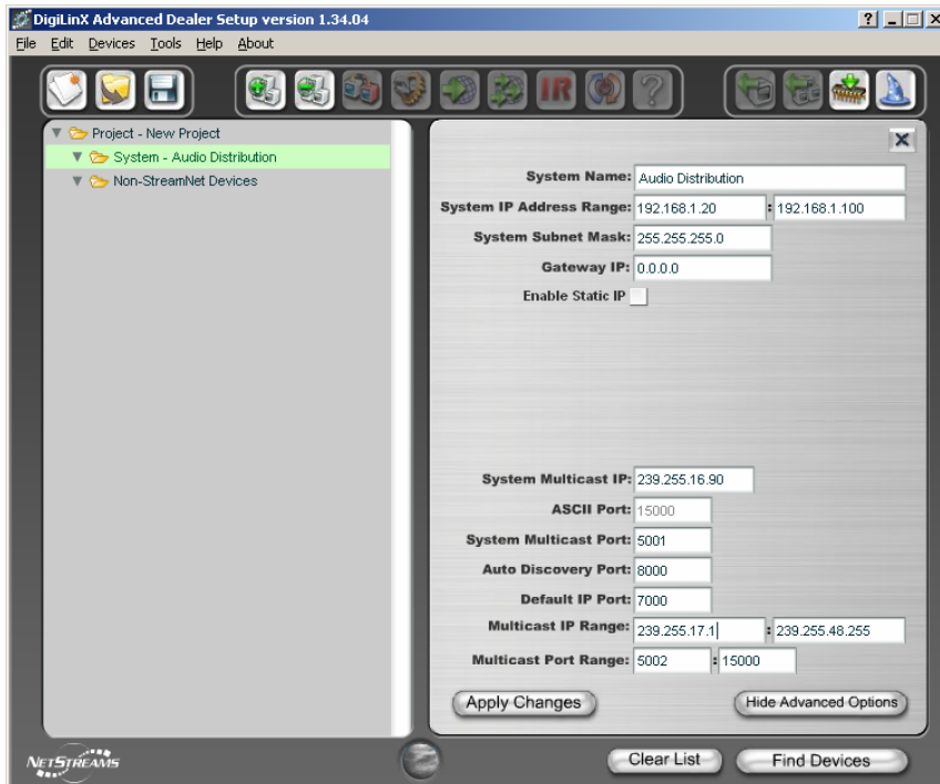
Figure 6 Building a DigiLinX IP Network (5 of 6)
