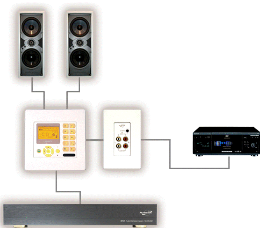
Figure 1 Local source connected to a Musica system
