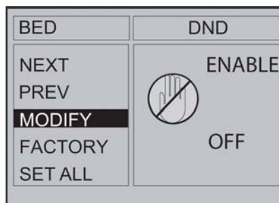
Figure 4-16 Giving the room the ability to toggle ON and OFF Do Not Disturb mode
